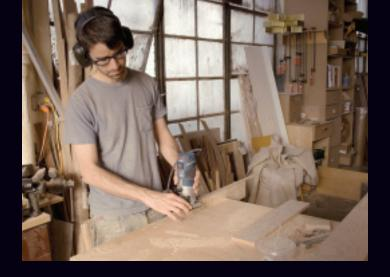
Left: Fairbank flush trim routing the edge of a veneered drawer face. The material core is plywood and must be veneered on all surfaces.
